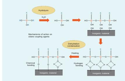
The inorganic group (R) of the silane molecule will hydrolyze to produce silanol, which forms a metal hydroxide or siloxane bond with the inorganic material. The organic group (X) of the silane molecule will react with the organic material to produce a covalent bond. As a result the organic material and the inorganic material are tightly bound together after heating.
